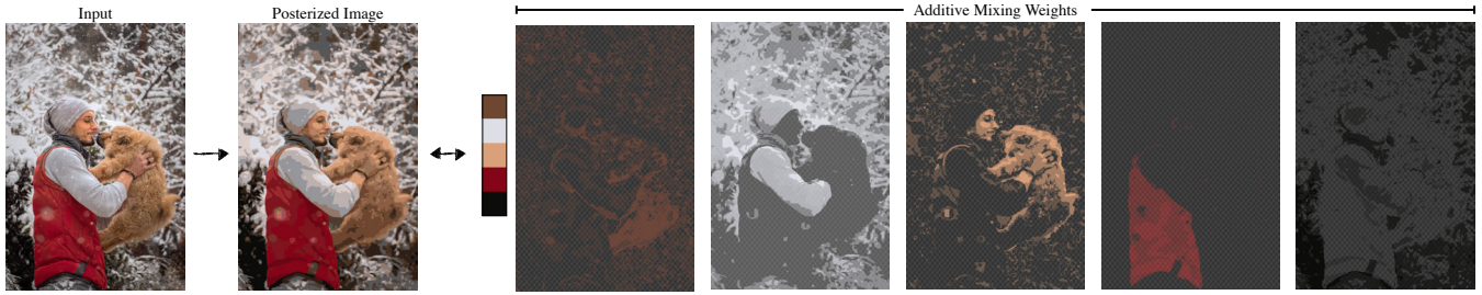
Figure 8: Visualizing the additive mixing weights for colors in the palette. These weights are computed before region boundary smoothing. Image ©Omid Armin
